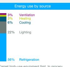
Target high-use equipment first. In grocery, upgrades to display cases, fans, and defrost controls could reduce refrigeration energy use by up to 30%. Routine maintnance, proper stocking, and carefully managed set points can contribute 10-15% savings.
